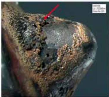
**Flow restriction, especially at maximum needle lift**
